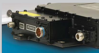
ARINC 781– consistent interfaces for fast maintenance.
